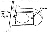
7. With a Phillips screwdriver, reach through the rear exhaust opening and remove the screw that attaches the cover to the dryer base. Carefully remove the cover and screw through the rear exhaust opening.
